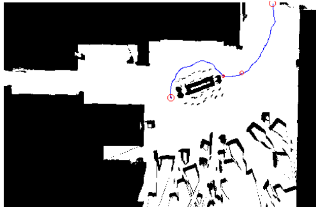
Figure 7. A pedestrian trajectory from the upper-right portion of the laboratory and around the table area. High-probability inferred subgoals (greater than 10% posterior probability) are displayed as red circles with areas in proportion to posterior probability.
